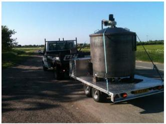
agricultural residue streams. The kiln can be transported from site to site on a small trailer. With feedstocks such as wood chips, rice husks, coffee husks, and other agricultural residues, users can utilize materials at hand.
