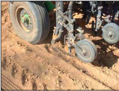
Biochar being banded in a Western Australia wheat field. Photo: P. Blackwell.
