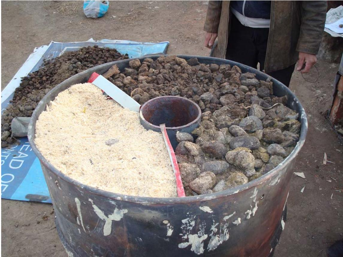
5. For a further trial the drum was partitioned into vertical thirds. One each was filled with sawdust, 'paddock' (winter camp, packed) manure and field dried manure. As before, the sawdust was not charred completely through, nor was the paddock manure. However, the field dried manure was well charred throughout.
