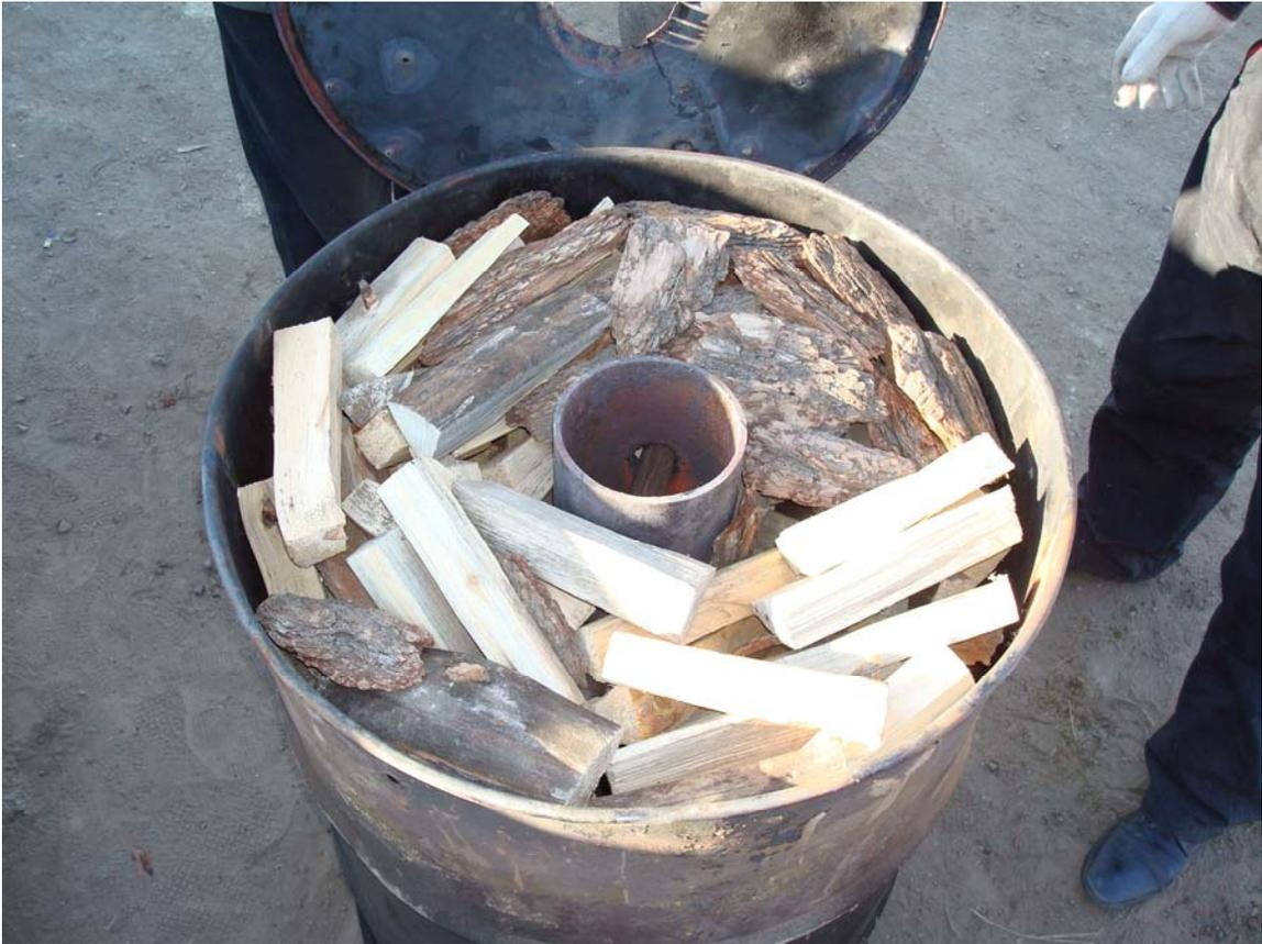
6. Another trial was run with a drum load of commercially available larch stove wood with a few pieces of thick larch bark. The wood and bark were well charred. A great deal of clean burning flame exited the top of the cowling during the burn indicating that there was insufficient O<sub>2</sub> entering the core at the height of pyrolysis to allow for complete burning of the p-gas there.
