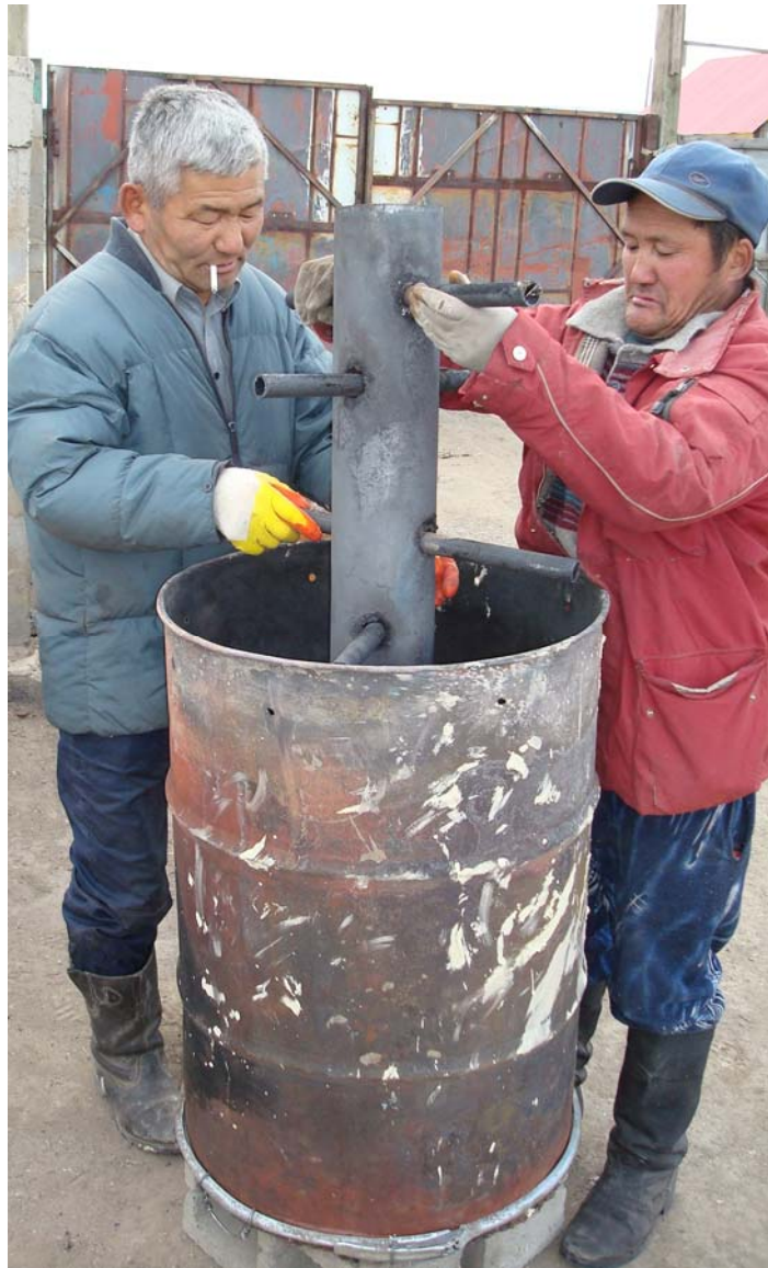
2. In this design gas ports in the core were enlarged enough to loosely hold horizontal, open ended hollow pipes (core lateral arms).
