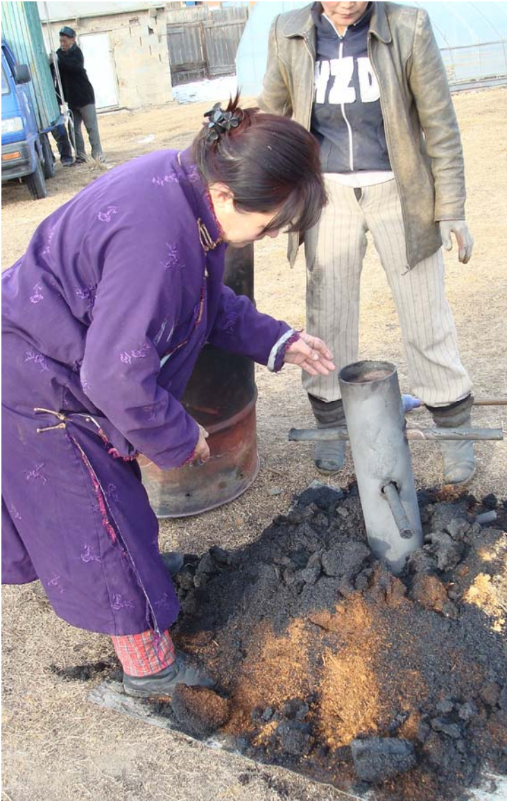
4. The design is insufficient to cause good charring throughout a load of sawdust because of the sawdust's strong insulation properties.
