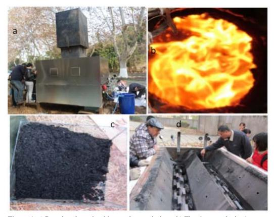
Figure 4. a) Running the unit with very low emissions. b) Flaming pyrolysis c) Biochar d) Examining the unit after running.
