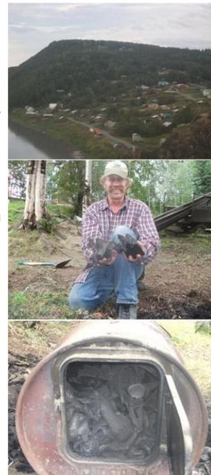
made to accompany biochar production with the generation of heat to be used at the NESFI farm facility. Additionally, a small scale continuous feed pyrolyzer prototype is being tested as NESFI.
