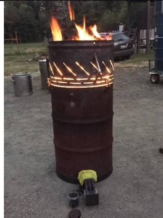
Making biochar in an engineered 55 gallon TLUD. Norman Baker and Paul Taylor. biochar-us.org/presentation/55gallon-tlud-progress-and-developments
