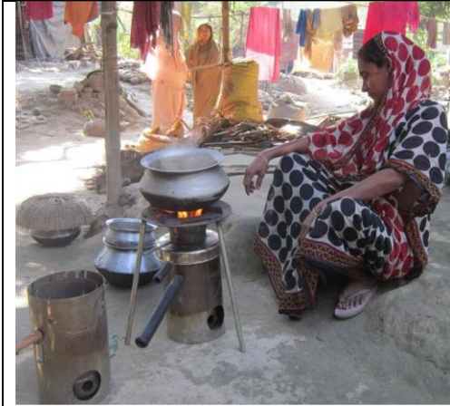
Champion model TLUD used to cook food and make biochar in Deganga, India. Paul Anderson (drtlud.com/deganga-tlud-project-2016)
