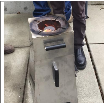
5kW TLUD Seachar stove at low power. Seachar.org
