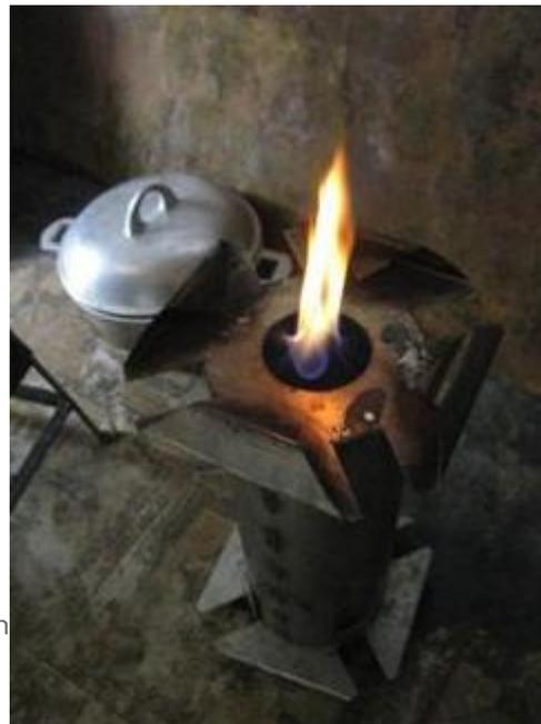
*Photo: The blue flame indicates that the Haiti Lucia stove is burning cleanly and efficiently; courtesy of World Stove*
