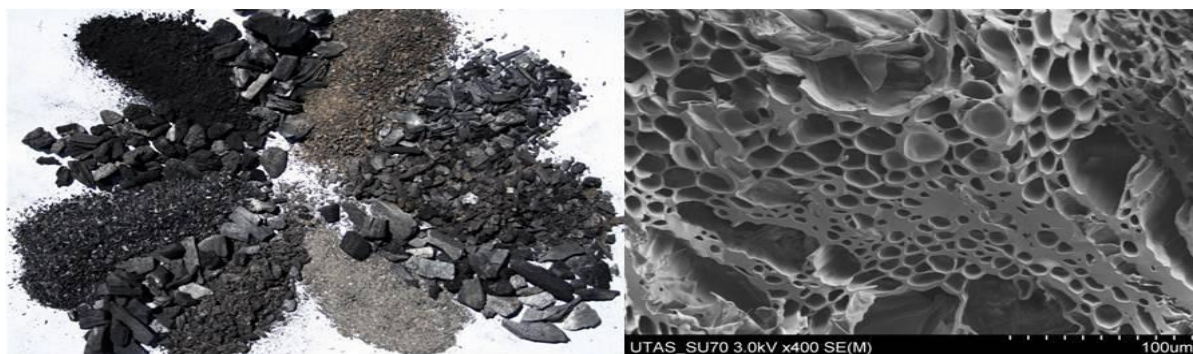
Biochar is a spectrum of materials made up of differing physicochemical properties. Note the well-defined pore structure in the scanning electron micrograph image on the right. Images courtesy of the UC Davis Biochar Database and biocharproject.org
