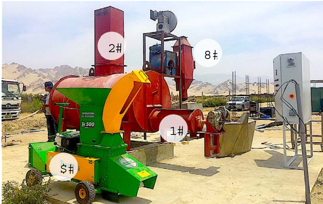
Figure 05. Integrated system from a pyrolyser of continuous production of fertilizers and spirulina. In the image the following phases are described (A) Biomass crusher, (B) entry of organic waste, (C) chimney for the conduction of gases, (D) exchanger for the recycling of heat for the drying of the microalgae and (E) use of CO 2 for the production of spirulina. Photo: Yngrid Espinoza.
