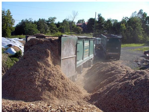
feedstock consists of wood waste, mostly from used shipping pallets and "clean" construction waste (i.e. wood not treated with heavy metals or other toxic substances). Brian and employee Alex English, who had previous experience with pyrolysis technology, have been inventing and modifying current hardware (and software!) to improve the efficiency and cleanliness of their continuous pyrolysis process and allow the production of biochar.
