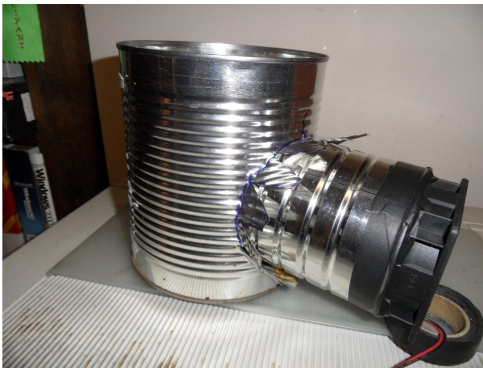
Figure 3: Attaching the fan-can to the larger can
