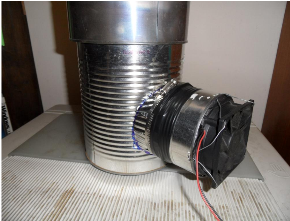
Figure 4: The completed Air Base – with a different fan-can attachment shown
