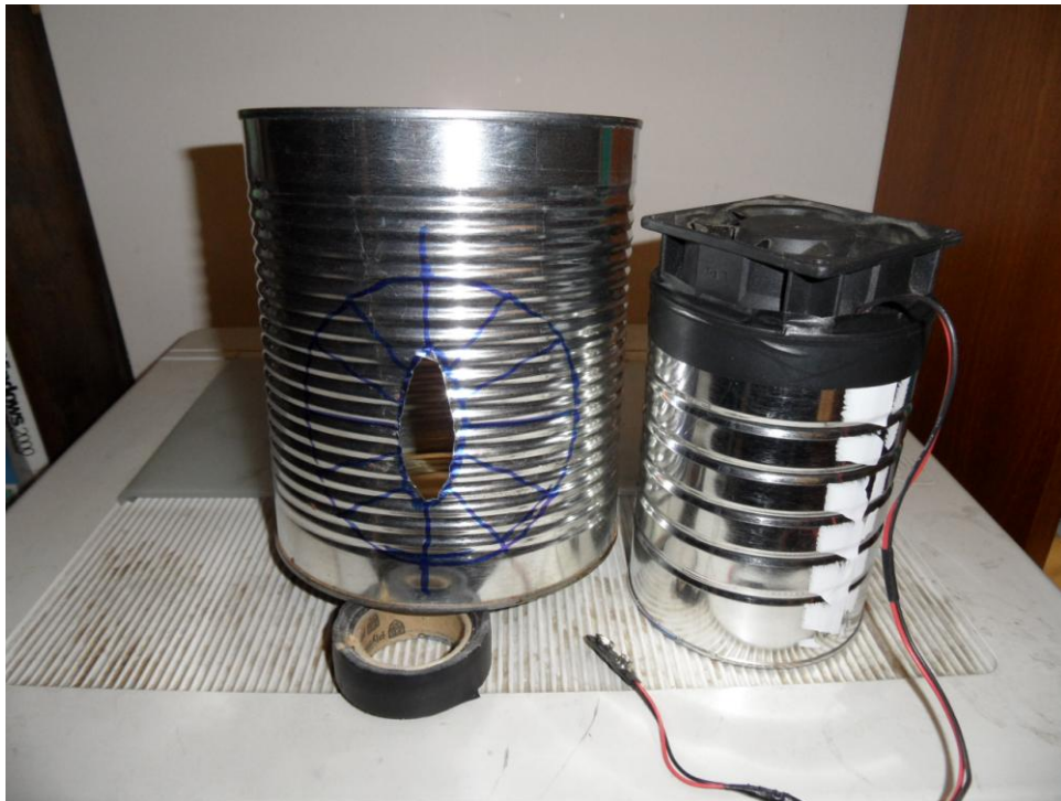
Figure 2: Layout of large can on left and finished "fan-can" on right
