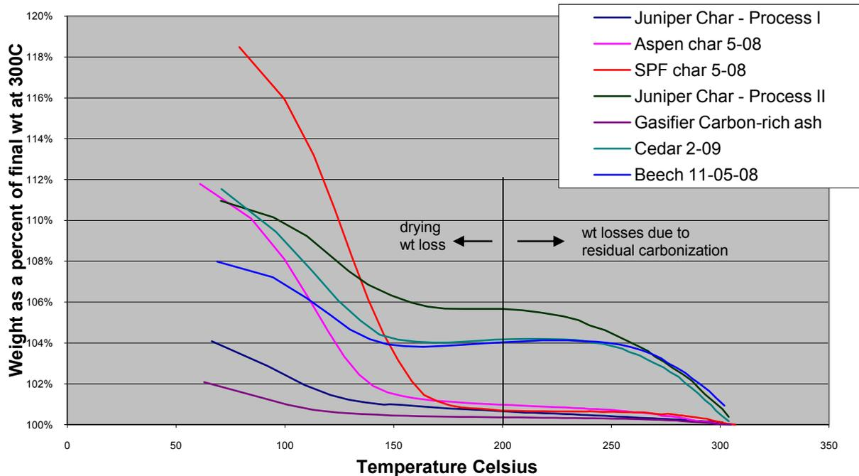
Prior to drying, the candidate char should be crushed and sieved to yield a coarse granular material, with granules between 1 and 5 mm in diameter. After the char is dried to approximately 200 degrees Celsius, it is cooled in a container with a sealed lid to avoid uptake of atmospheric moisture. Once cooled, a weighed clean dry tomato paste can is filled about one half way with dry granular char and weighed again.
