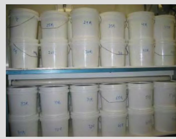
Fig. 1: Sealed buckets used for the char-C turnover experiment. The NaOH solution in the bucket traps the CO 2 released during char decomposition.
