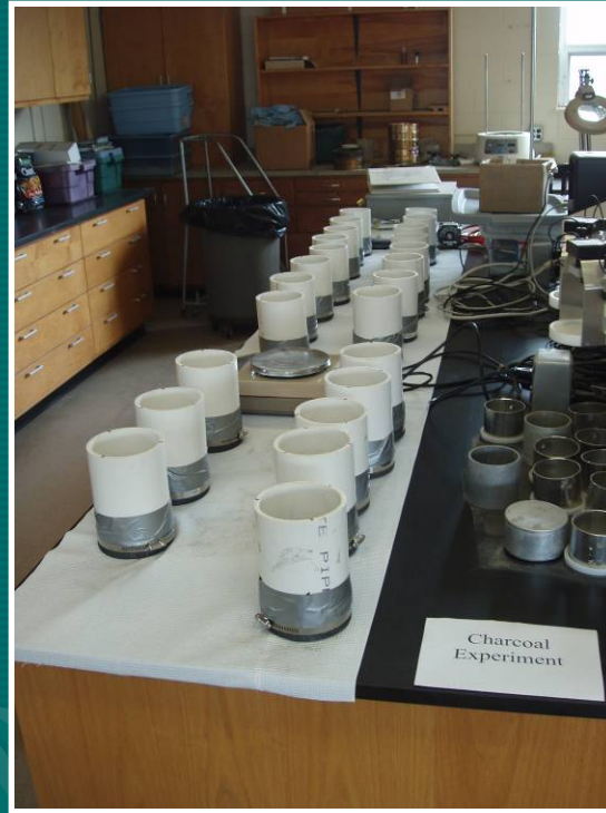
Columns with soil and biochar (SOC, CO 2 , aggregates, and strength measured)
