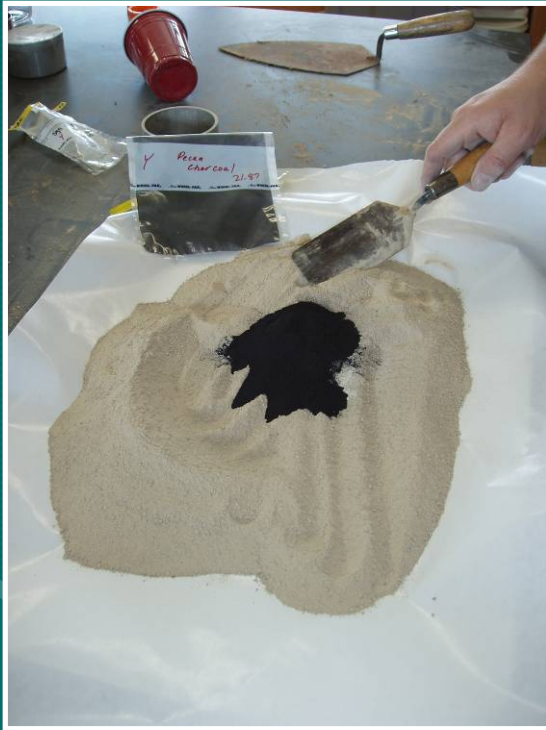
Creating Norfolk soil + biochar mixtures (0, 0.5., 1.0 and 2.0%)
