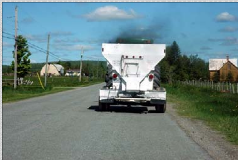
Transporting an unprocessed, fine biochar material to the field, applying and incorporating it in St-François-Xavier-de-Brompton, Québec. Both images show biochar blowing off. Photos courtesy of Blue Leaf, Inc., www.blue-leaf.ca .
